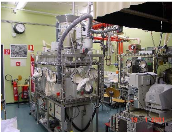
Fig. 1a) Revaporisation device with lead-shielded oven, diluter & filter with \gamma -detector above glove-box
