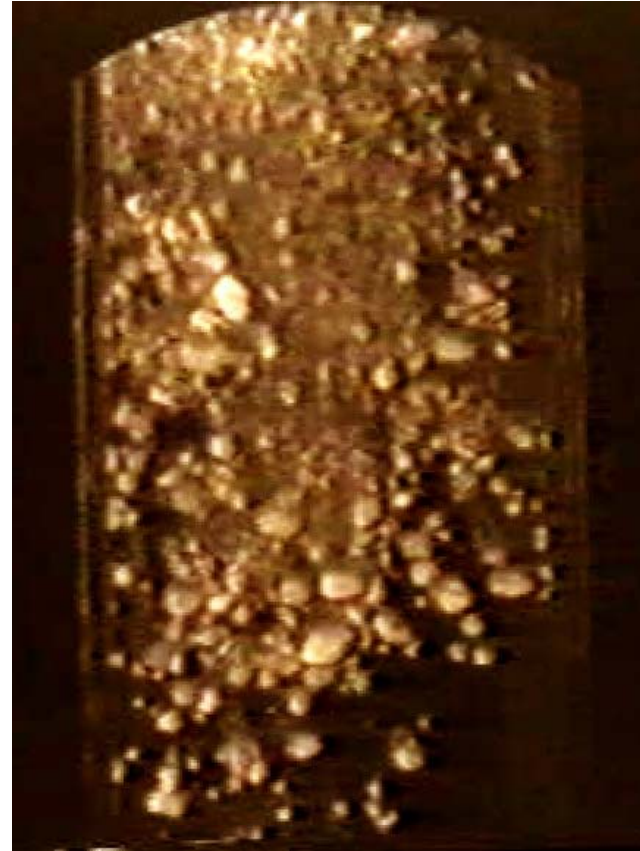
Alumina melt mixing in K-57 (CANON). Viewing area 10 by 20 cm
