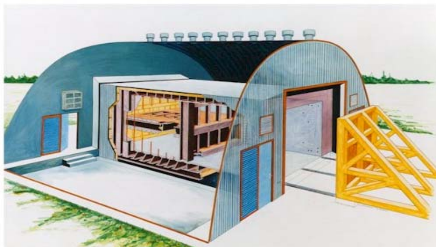
Figure 6: Large-scale Vented Combustion Test Facility configured for Multi-Chamber PAR Tests (rear top/bottom chambers on left, front chamber on right)
