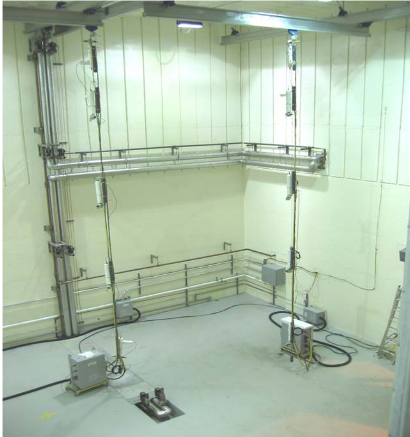
Figure 2: Large-Scale Containment Facility (LSCF) used to perform helium/air/steam mixing experiments
