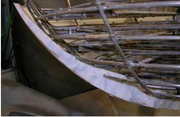
Figure 15: Post test view of crust in LIVE-L1.
