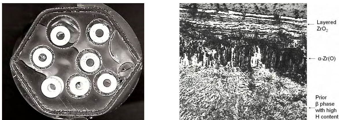
Fig. 27: Cross section of CODEX-CT-2 bundle (left) and piece of cladding with layered oxide scale (right)
