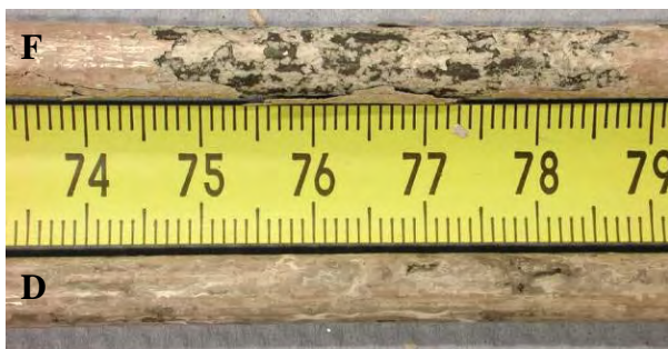
Fig. 14: QUENCH-12, the withdrawn solid corner rods D and F (E110) revealed breakaway oxidation with intensive spalling of oxide scales
