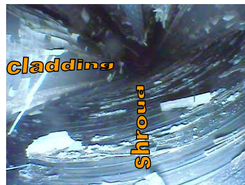
Fig. 15: QUENCH-12, videoscope inspection of breakaway effect at the 650 mm elevation. Cladding: E110, shroud: E125 alloy
